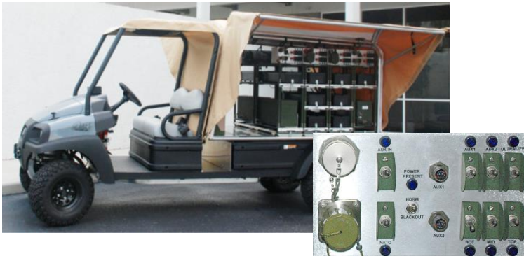
A Commercially Available, 4x4 Utility Vehicle Is Modified into a 9 kW Self-Propelled Power Generation System with Modular Mobile Charging System (MCS) Payload
