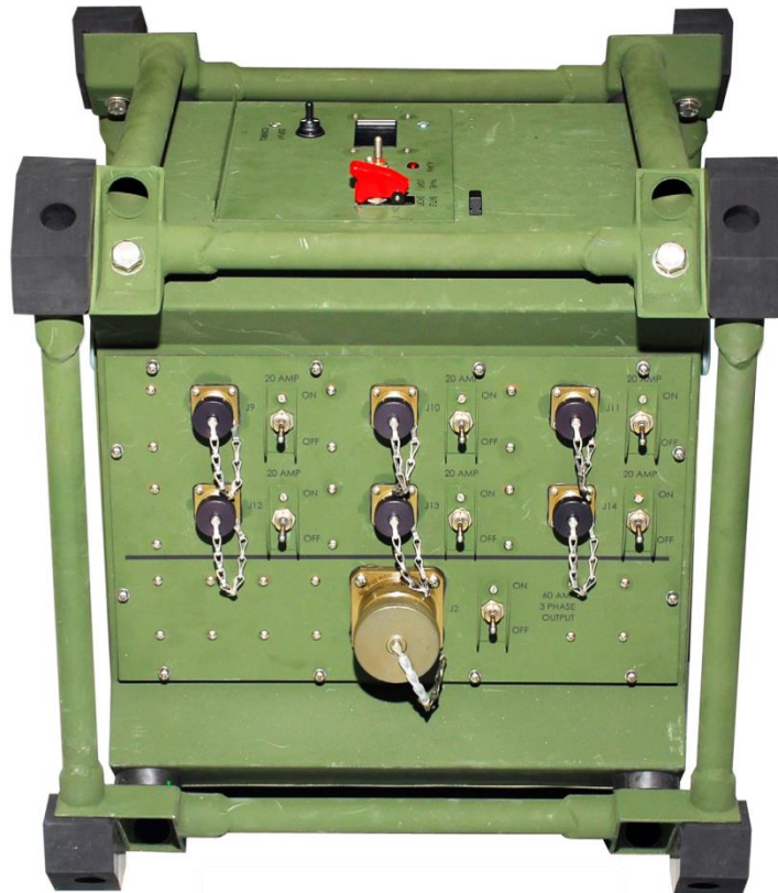
I40 Power Distribution Center 60 AMPS
